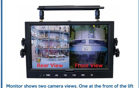
Monitor shows two camera views. One at the front of the lift truck and another mounted facing the rear. Up to 4 cameras can be paired to one monitor.
